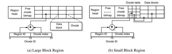
Figure 3. Region structure and data layout.
