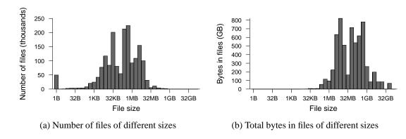
Figure 1. Data distribution in a large high-performance distributed storage system (data courtesy of LLNL)
